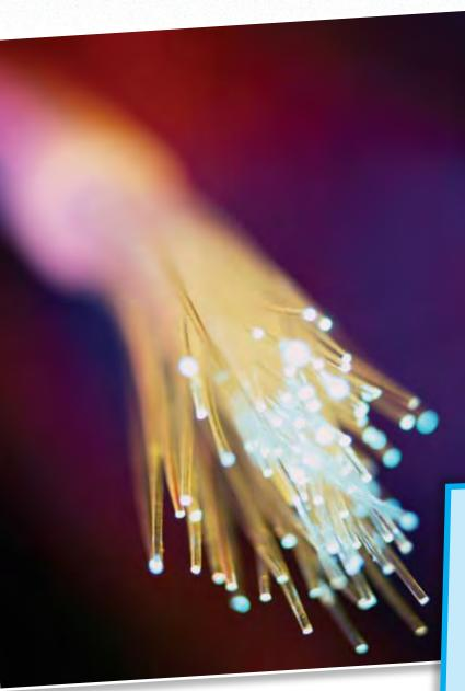
Optical fibers are thin filaments of glass that are used as communication cables. They use light beams to transmit audio, video, and data. They work on the principle of total internal reflection. They have enormous data carrying capacity at low-cost. In 1930 Heinrich Lamm, a German student, became the first person to use optical fibers to carry an image.
