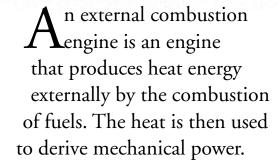
The heat produced by the external combustion engine heats a working fluid, such as water. Steam engines and Stirling cycle engines are examples of external combustion engines.
