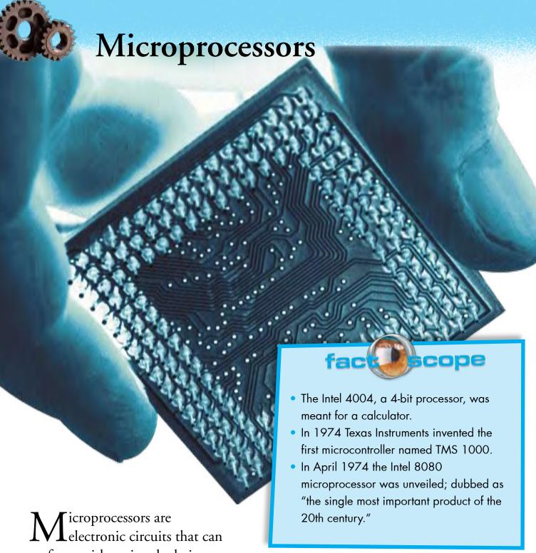
Microprocessors are electronic circuits that can perform arithmetic calculations and control programs with great accuracy. It is often referred to as a logic chip or master chip. It acts as an engine of the computer. The world's first single chip microprocessor, Intel 4004, was introduced by Intel Corporation in 1971.
